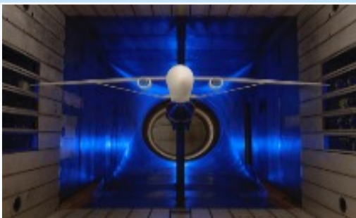
Transonic Truss-Braced Wing 5-10% fuel burn benefit
